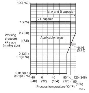
Figure 1. Working Pressure and Process Temperature
