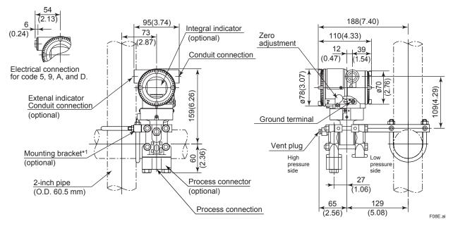
\*1: A transmitter with SST housing is not applicable for mounting to horizontal 2-inch pipe.
